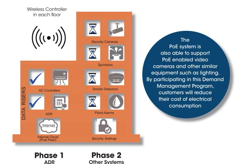
Communication consists of Power over Ethernet (PoE) data cables. The data cables incorporate a network hub on each floor that communicate to the z-wave controllers and also provide them with power. This greatly reduces the cost of the installation as many of the areas may not have available electric outlets and a PoE system does not require them.
